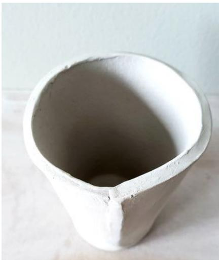
**Uneven slab:** Using an uneven slab will result in a pronounced and weak seam. Difference in thickness can also cause cracks during drying and firing. It also stands out as a mismatch, doesn't look as good.
